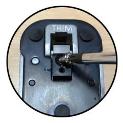
**STEP 2**Loosen the screw of the trimming blade.
